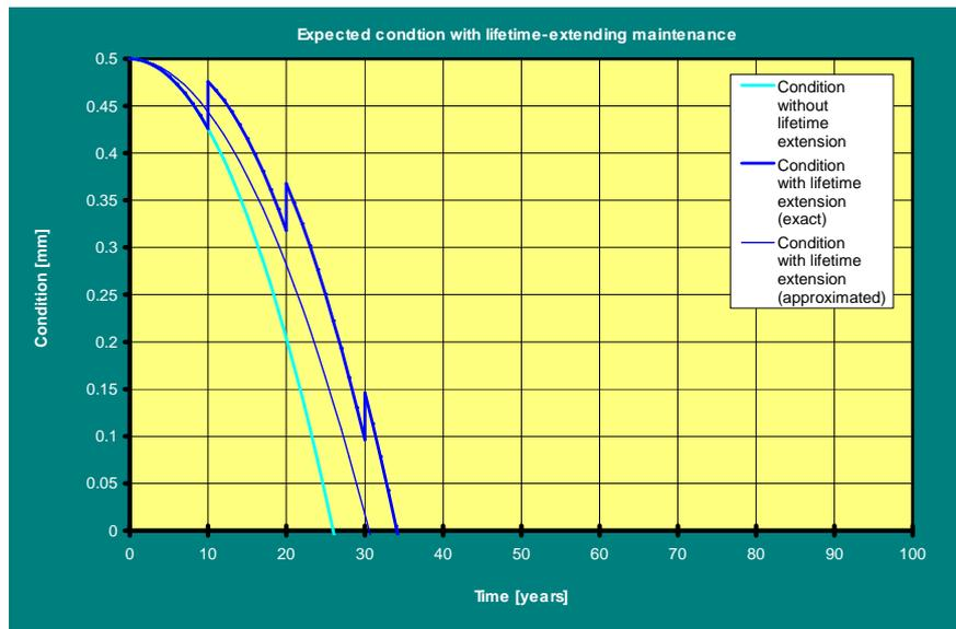
Figure 3. Example of lifetime-extending maintenance with non-repeating propagation curve.
