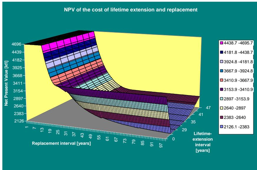
Figure 7. NPV of the expected cost of lifetime extension and replacement for the slabs.
