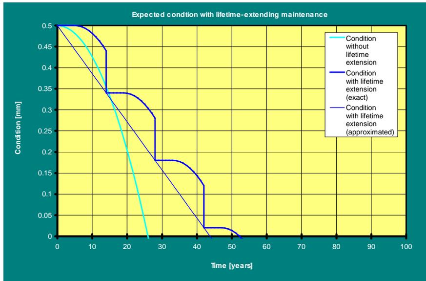
Figure 10. Expected condition with and without lifetime extension for the joints.
