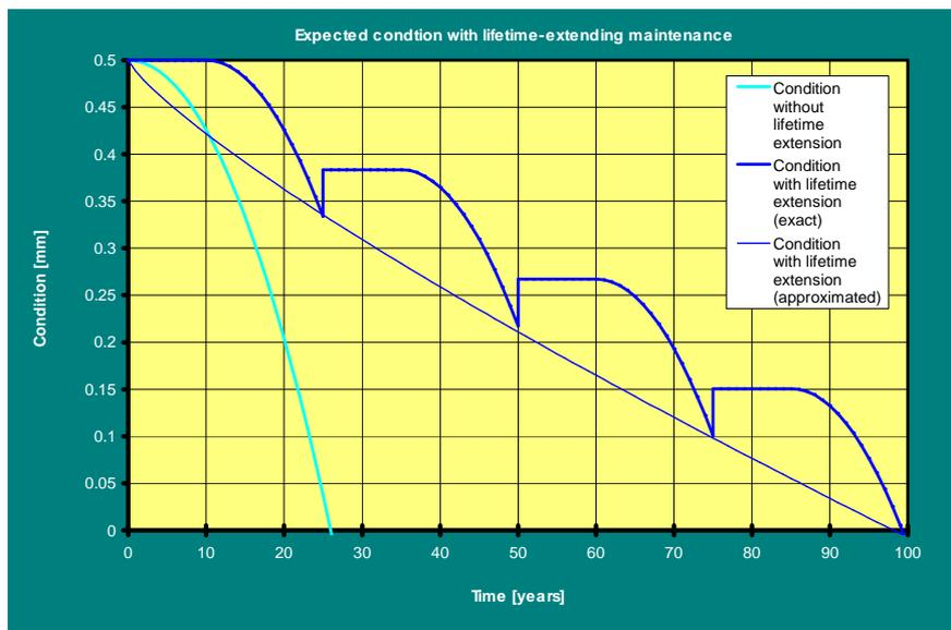
Figure 2. Example of lifetime-extending maintenance with repeating propagation curve.
