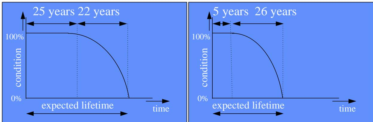
Figure 5. Expected deterioration without lifetime extension for the slabs (left) and the joints (right).
