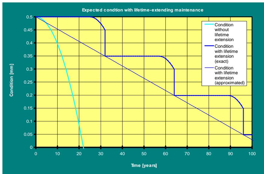
Figure 8. Expected condition with and without lifetime extension for the slabs.
