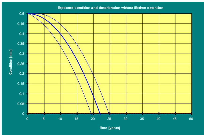
Figure 6. Expected condition without lifetime extension for the slabs including the 5th and 95th percentile.
