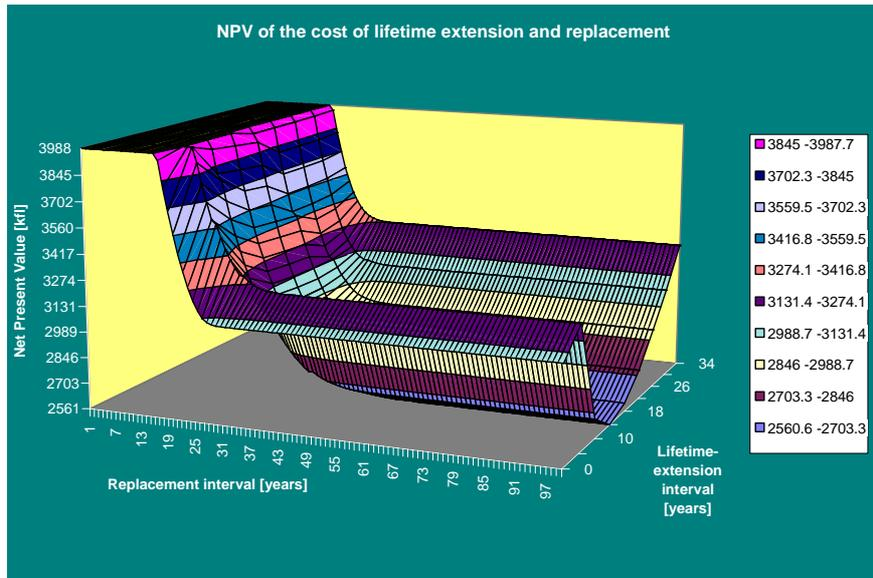
Figure 9. NPV of the expected cost of lifetime extension and replacement for the joints.
