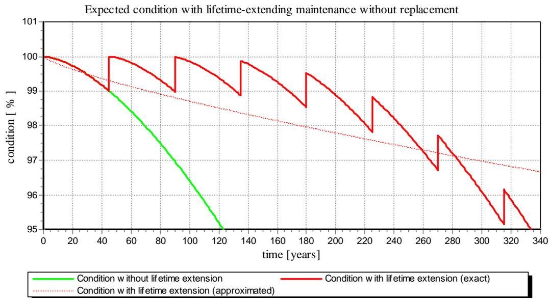
Figure 8 Optimal maintenance interval of 45 years
