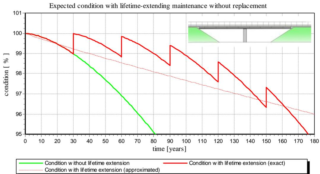
Figure 7 Optimal maintenance interval of 30 years
