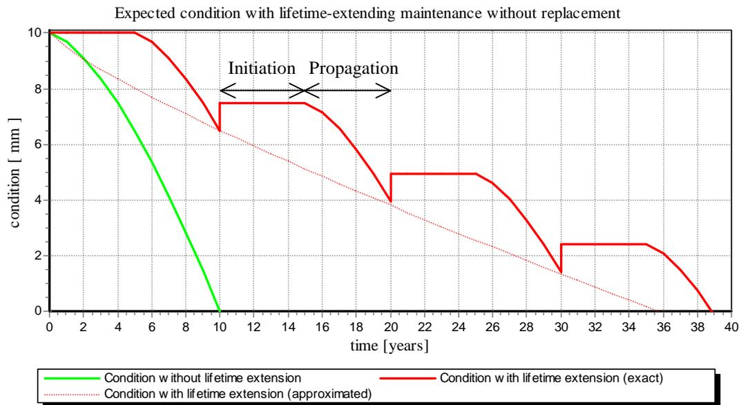
Figure 1. Example of lifetime-extending maintenance with repeating propagation curve.
