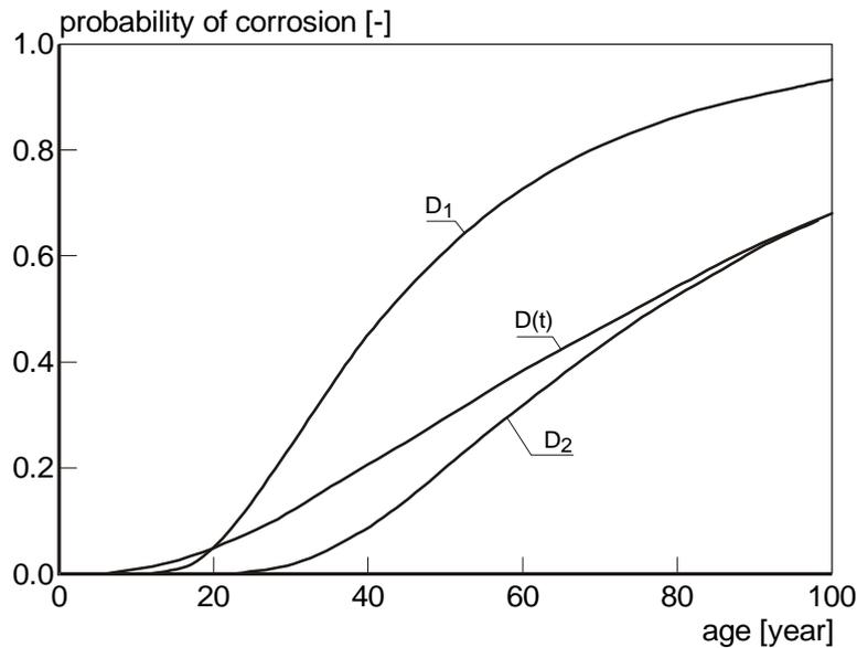
Figure 3 Example of probability of corrosion due to chloride ingress.
