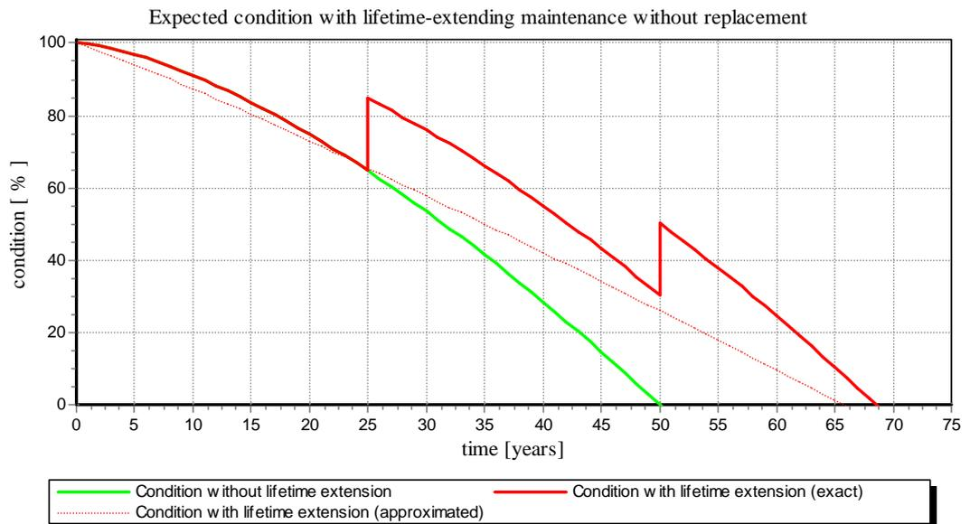
Figure 2. Example of lifetime-extending maintenance with non-repeating propagation curve.
