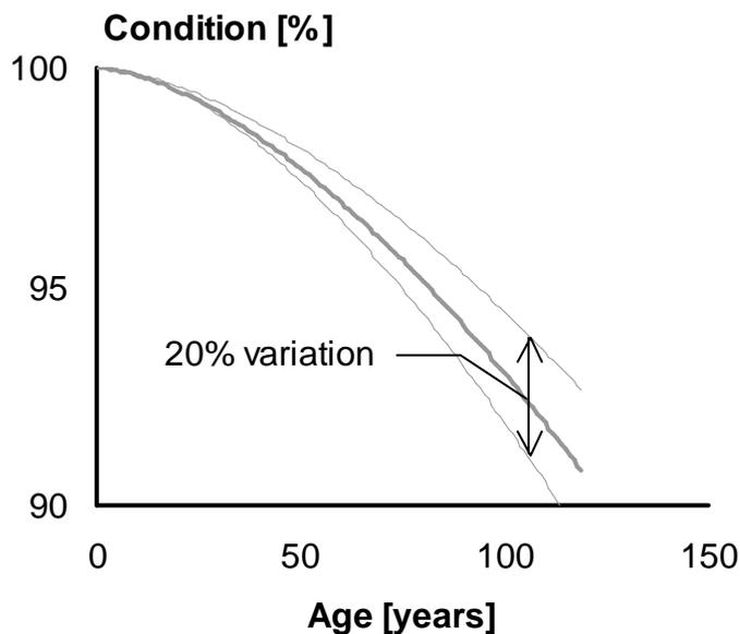
Figure 4 Condition model according to the experience at the Ministry of Public Works. The 20% variation holds for the condition at the time at which the expected condition equals the failure level of 95%.
