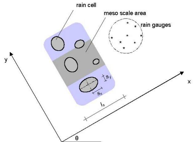
Figure 5. Schematic representation of spatial structure of rainfall including rain cells and meso scale areas or rainstorms (adapted from Willems 2001), where  $s_x$  is spatial extent of rain cell in moving direction,  $s_y$  is spatial extent of rain cell perpendicular to moving direction,  $\theta$  is average moving direction of rain cells,  $l_s$  is spatial extent of rainstorm (meso scale area) and  $i$  is number of rain gauges.
