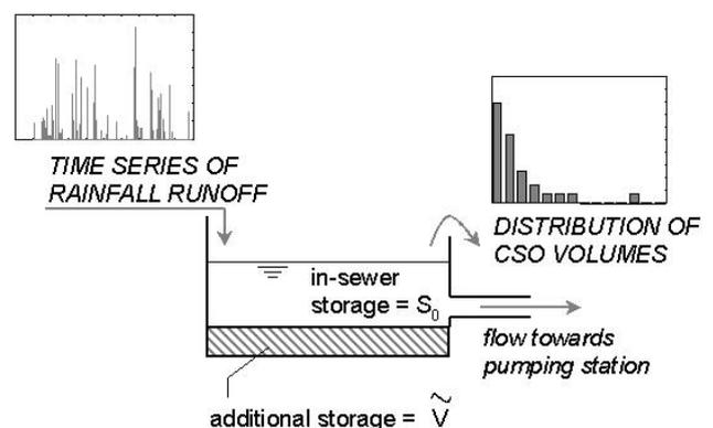
Figure 2. Schematic representation of the decision problem: enlarging in-sewer storage capacity in order to prevent CSOs (optimal storage volume = in-sewer storage ( $S_0$ ) + additional storage ( $\tilde{V}$ )).
