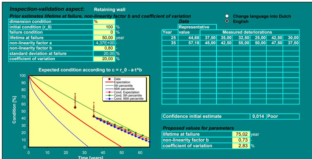
Figure 6. Inspection validation on representative values, reference steel thickness: 4 mm.
